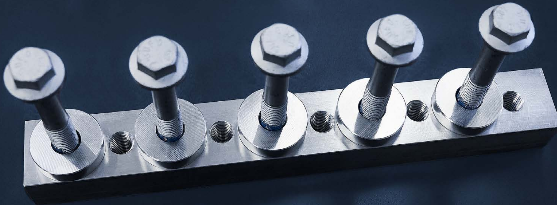
Test materials lined up for friction testing.
