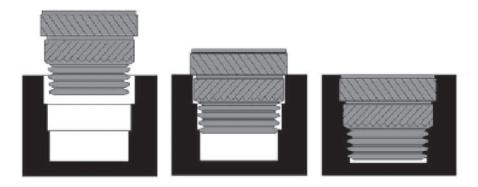
TRI-STEP™ Inserts provide the ease-of-location and hole-centering benefits of a tapered insert, while eliminating the inherent drawbacks of a tapered design.
