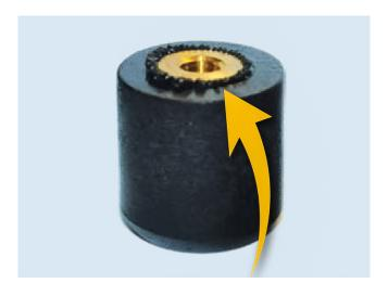
Tapered inserts often produce plastic flash, resulting in secondary de-burring processes and added costs.
