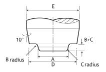
Punch material 1% C/Mn Steel (Silver Steel). Water quench pilot end from 820°C, Temper at 260°C.
