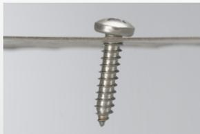
Standard type ST screws lean over as the screw tends to align with the helix angle of the thread. Stripped threads or loose assemblies result.
