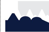
The MATHread® unique male thread 'rolls' over the first thread in the female thread crest.
