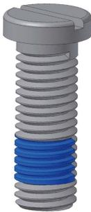
PSM can offer a wide range of thread locking and sealing solutions, eliminating the need for secondary locking devices. Nylon Patch when applied, is permanently fused onto the thread of the screw or threaded component. The patch increases the prevailing torque and provides excellent vibration resistance, allowing the screw to be locked in any position when assembled.
