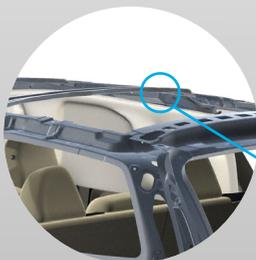
Clip Screw pre-assembled in inflatable curtains delivered by Autoliv and finally assembled by Volvo Car Corp.
